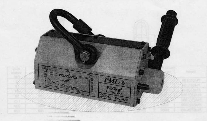
Principles: Model PMQZQ Permanent Magnet Lifter has strong magnetic path produced by Nd-Fe-B magnetic materials. On and Off of the magnetic path is controlled by turning the manual handle. PMQZQ permanent magnetic lifters have magnet as power, and its lifting power will never weaken.
